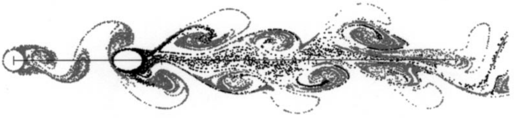
Figure 16. A particle simulation of the flow field around an elliptical cylinder downstream of a circular cylinder at Re = 141 (based on the circular cylinder diameter) and g^* = 3.0 (based on the largest dimension of the elliptical cylinder). The superimposed bar scale is 15 times the length of the largest dimension of the elliptical cylinder.
